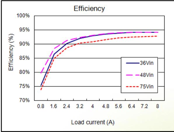
Figure 1: Efficiency ( $T_A = 25^\circ\text{C}$  or  $77^\circ\text{F}$ )
