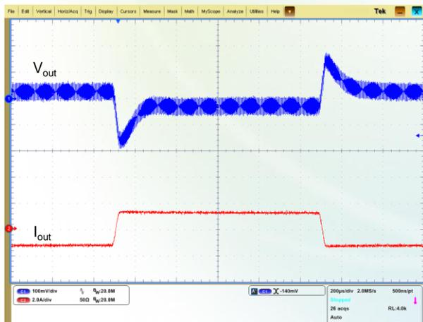
Figure 13: Output voltage dynamic response
