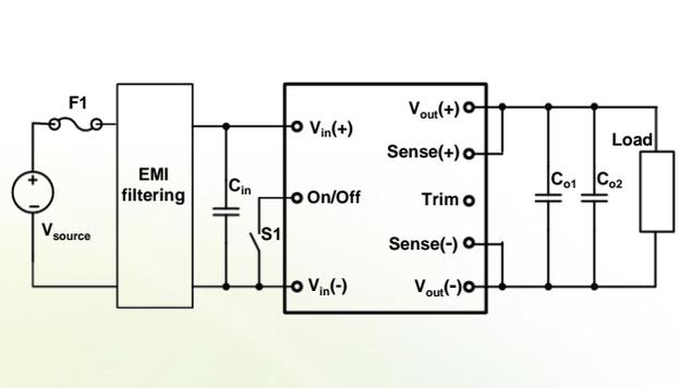
Figure 6: Typical circuit applications
