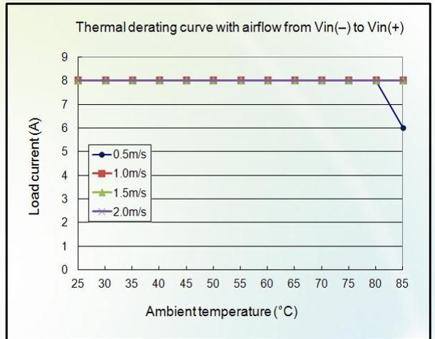
Figure 4: Thermal derating with airflow from  $V_{in(-)}$  to  $V_{in(+)}$  ( $V_{in} = 48\text{ V}$ ;  $V_{out} = 12\text{ V}$ )
