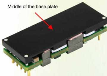
Figure 21: Thermal test point
