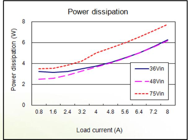
Figure 2: Power dissipation ( $T_A = 25^\circ\text{C}$  or  $77^\circ\text{F}$ )
