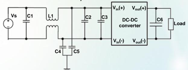
Figure 20: EMC test set-up diagram
