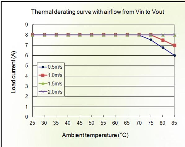
Figure 3: Thermal derating with airflow from  $V_{in}$  to  $V_{out}$  ( $V_{in} = 48\text{ V}$ ;  $V_{out} = 12\text{ V}$ )
