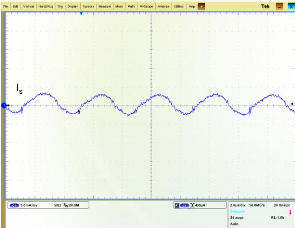
Figure 7: Input reflected ripple current (for point A in the test set-up diagram,  $V_{\text{in}} = 48\text{ V}$ ,  $V_{\text{out}} = 12\text{ V}$ ,  $I_{\text{out}} = 8\text{ A}$ )
