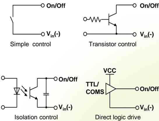
Figure 15: various circuits for driving the On/Off pin
