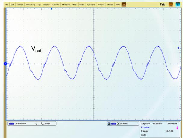
Figure 8: Output voltage ripple (for point B in the test set-up diagram,  $V_{\text{in}} = 48\text{ V}$ ,  $V_{\text{out}} = 12\text{ V}$ ,  $I_{\text{out}} = 8\text{ A}$ )
